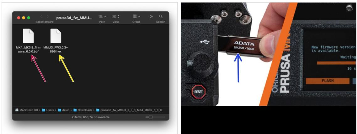
**⚠️ IMPORTANT!!!** Before you proceed further; There are two firmware files. One is for the printer. The other one is for the MMU3 unit. Both needs to be flashed to the respective device.
