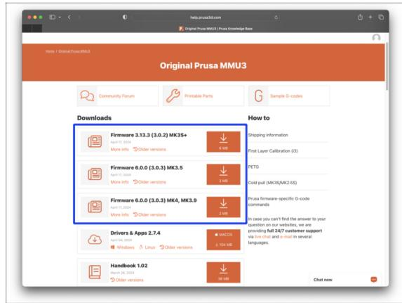
**⚠** You will need to update both the firmwares for the printer as well as the MMU unit. Use only a combination of the newest firmware versions for both devices together.
