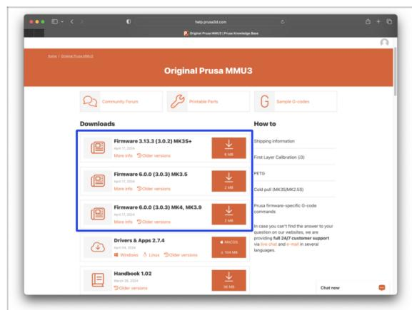
**⚠** You will need to update both the firmwares for the printer as well as the MMU unit. Use just the newest firmware versions together.
