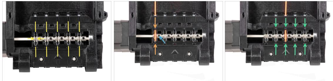
**⚠ WARNING:** this step is crucial in order for the MMU unit to work properly! Please check your pulley alignment multiple times!!!
