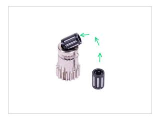
Insert both bearings into the gear. Be aware that bearings can slip out during assembly.
