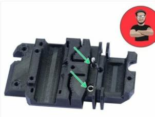
**⚠️ For the following nut insertion USE A SCREW. THAT'S AN ORDER!!!** Seriously, use a screw to pull the nuts in, both have to be properly seated in the X-carriage.
