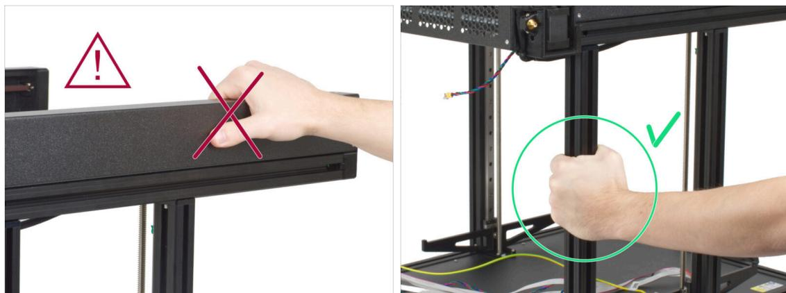
**⚠ Never lift or move the printer by using the upper metal flanges. You can damage the LED lights hidden inside.**
