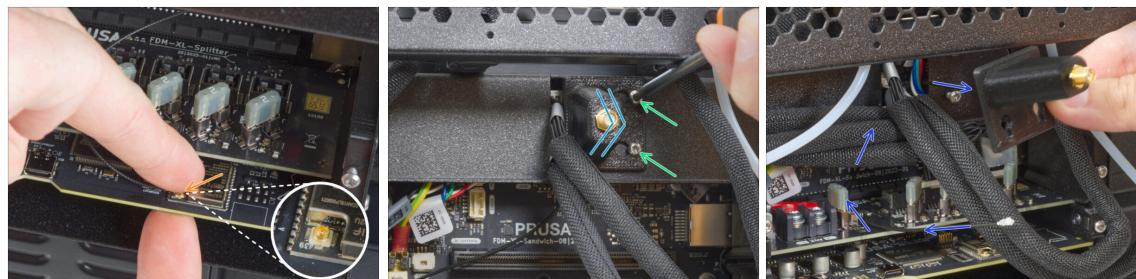
① If you have the antenna on the side of the printer -> **remove the cover** and proceed to the next step.
