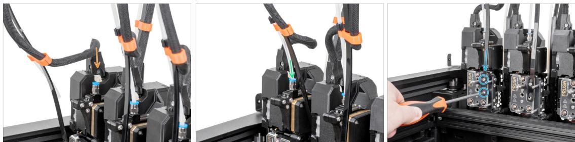
⚠ Check that the cable bundle is not twisted!
