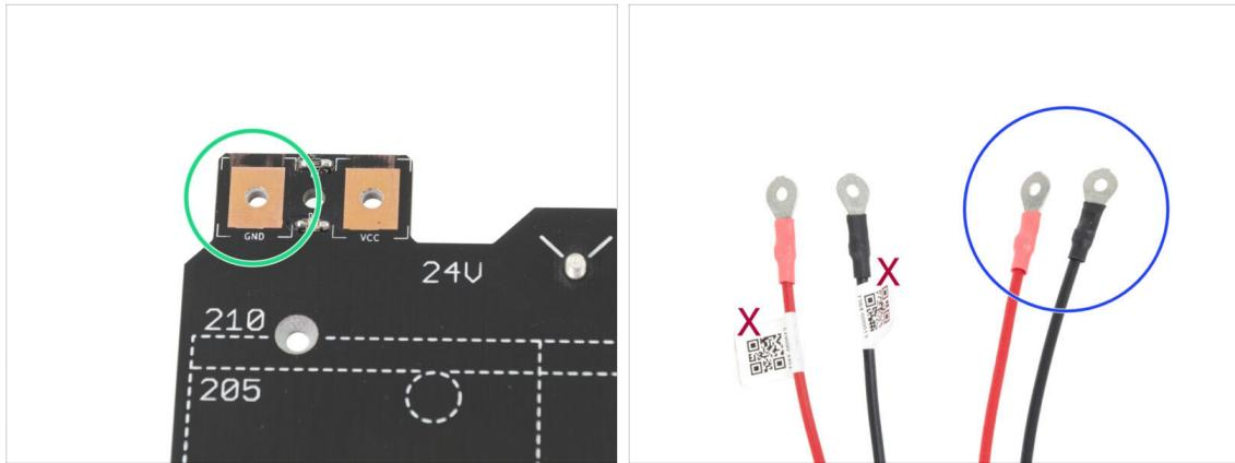
◆ Follow the polarity markings on the heatbed:
