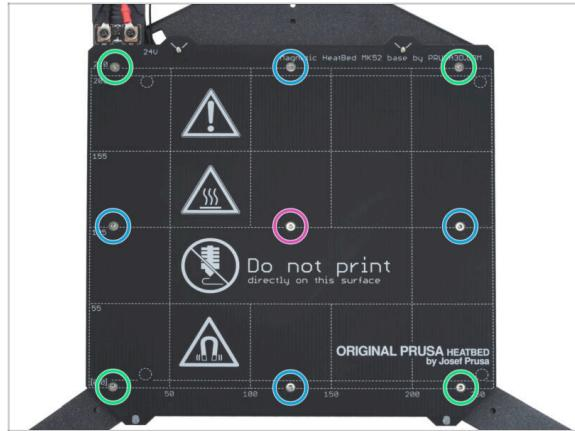
⚠ **IMPORTANT:** The heatbed must be tightened in a specific order. Repeat the sequence multiple times, ensuring the final tightening after at least two rounds.
