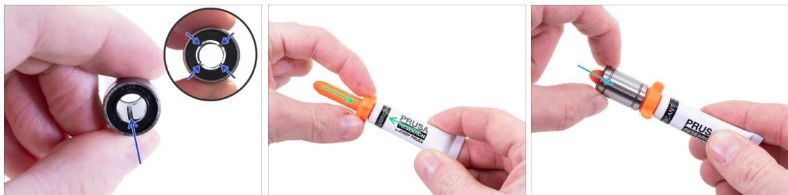
➊ Use any piece of fabric as a pad to protect your working surface from grease.
