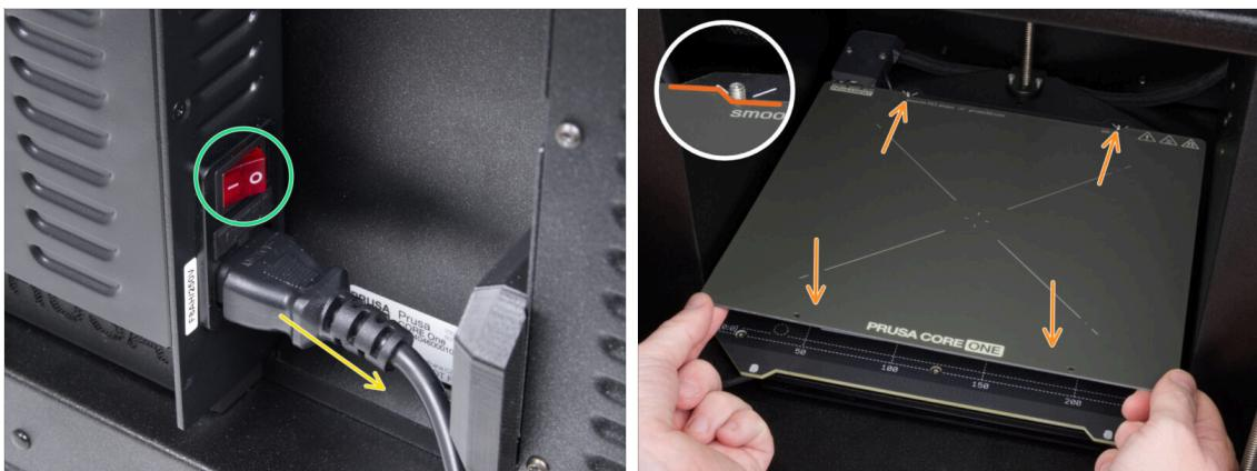
⚠ Before you begin, make sure the printer has cooled down to ambient temperature.
